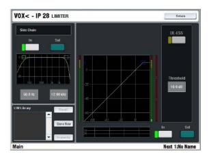
This is the last of three dynamics processors available on every input channel. It can be used either as a 'brick wall' limiter to stop the threshold level being exceeded or as a de-esser to filter out the sibilance of a vocal source.
